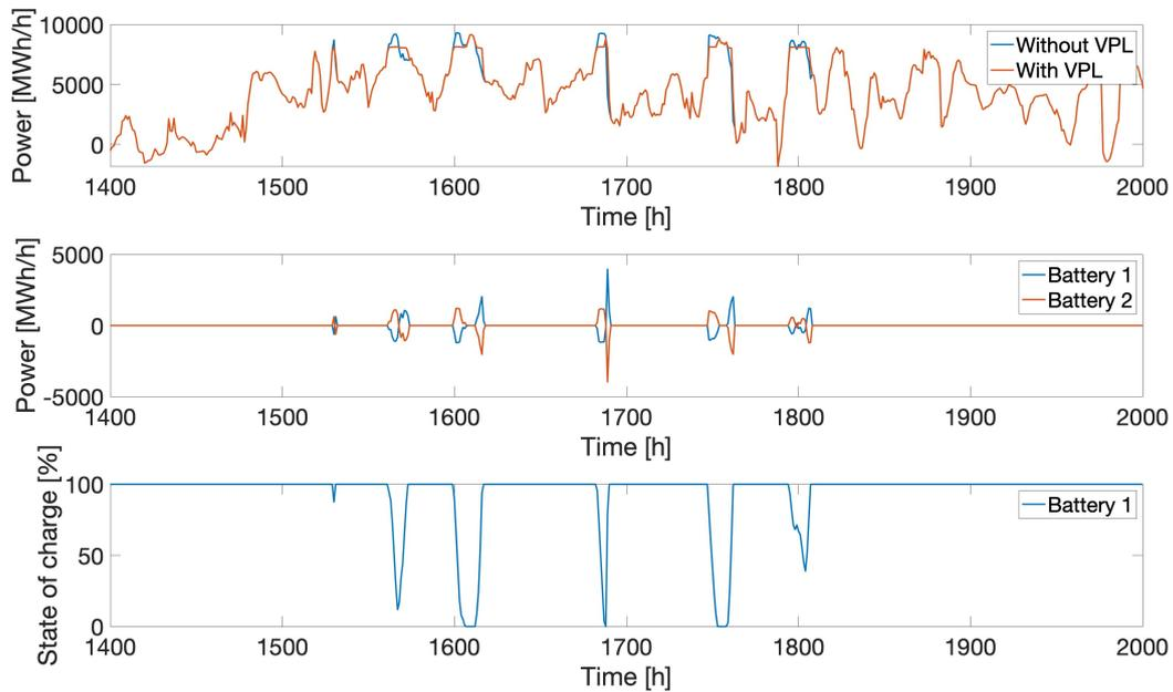
Figure 39: *The upper graph shows active power transfer across BZB2 both with and without VPL4 for a chosen period of time. The middle graph shows active power for the BESSs in VPL1 for the same chosen period of time for scenario Electrification dispatchable. The bottom graph shows the state of charge for the demand side BESS.*
