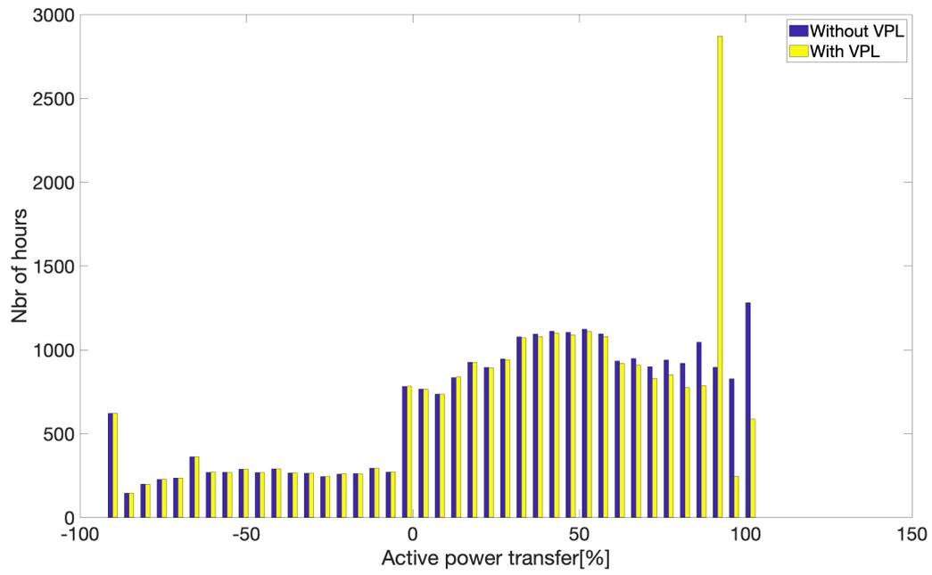
Figure 42: *BZB4 loadings both when VPL8 is connected and when it is not connected for scenario Electrification dispatchable.*
