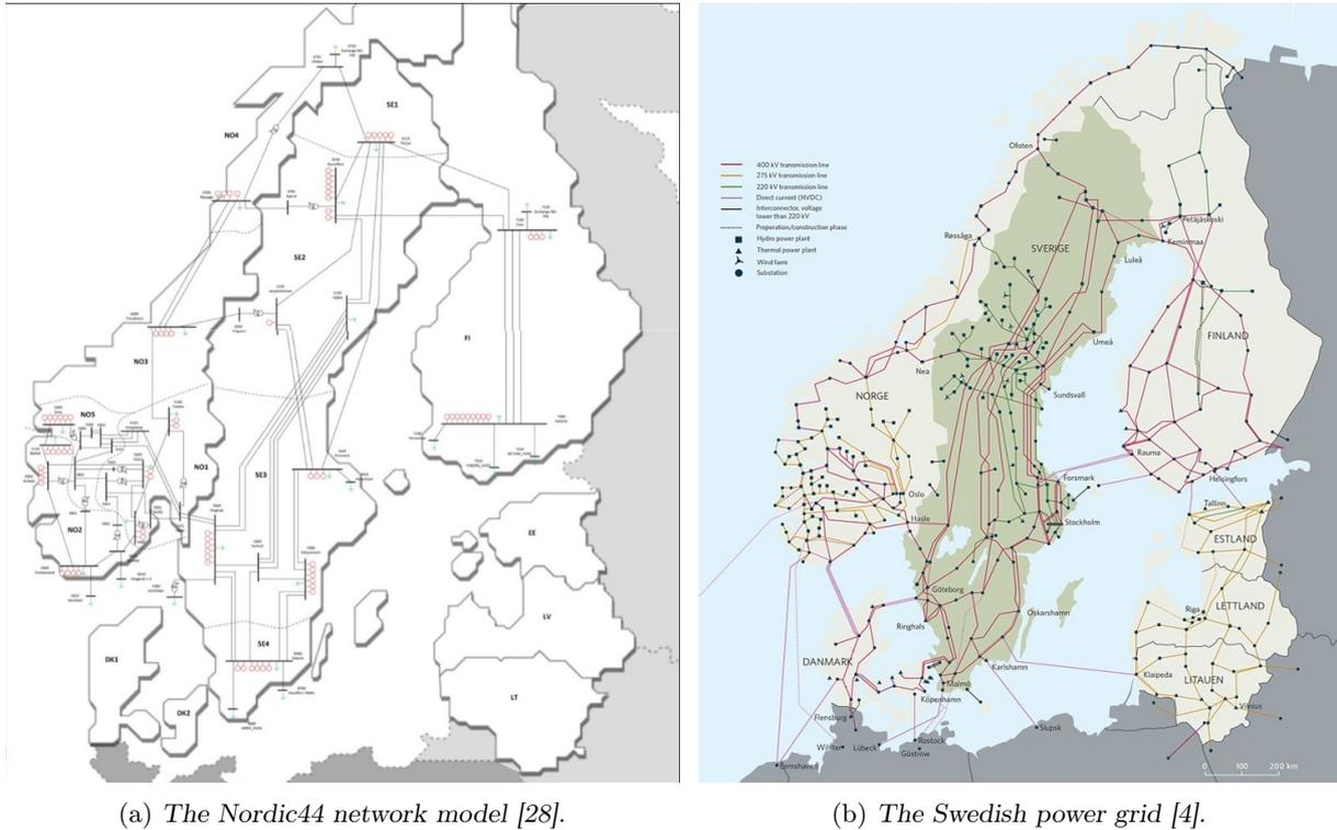
Figure 12: Shows how the transmission grid is modelled in the Nordic44 model and what the real transmission system looks like in the Scandinavian area.
