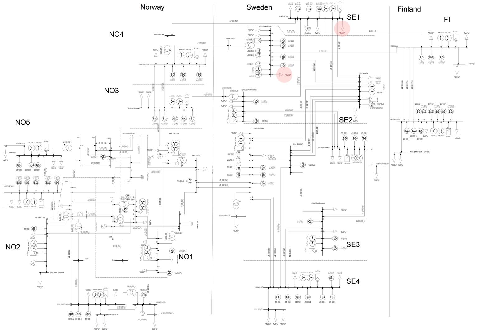
Figure 16: *The Nordic46 model. Wind power, solar power and new synchronous generators are added. HVDC links are updated. The number of loads on each bus is adjusted to 2. An extra load can be found on Porjus and Grundfors representing VPL1, marked with red circle. The bidding zones are updated to match the real ones.*
