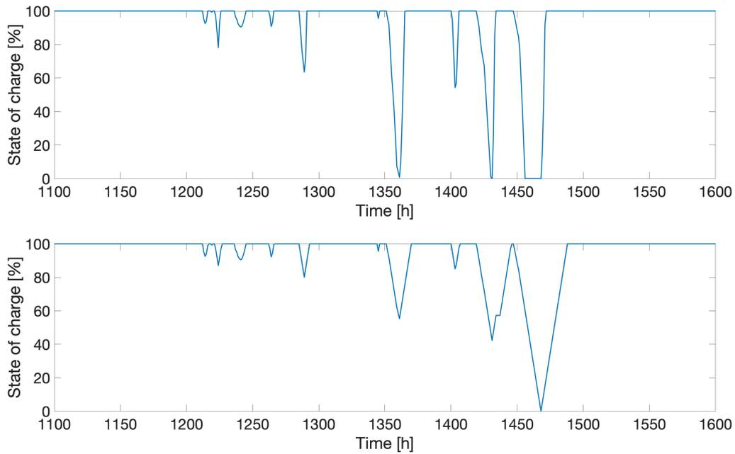
Figure 31: *The state of charge of the demand side BESS for VPL1. The upper graph represents the state of charge when the BESS system has an unlimited power rating, and the lower graph shows when the BESS has a limited power rating of 250 MW. The rate of changes in state of charge is lower when the power rating is limited.*
