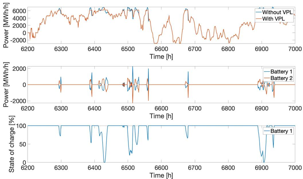
Figure 41: *The upper graph shows active power transfer across BZB4 both with and without VPL8 for a chosen period of time. The middle graph shows active power for the BESSs in VPL1 for the same chosen period of time for scenario Electrification dispatchable. The bottom graph shows the state of charge for the demand side BESS.*
